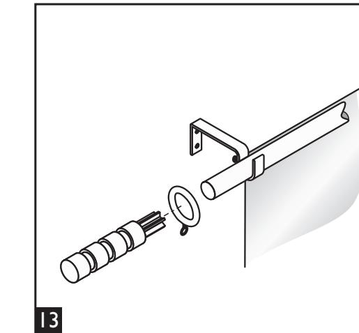
Note: To ease with pushing finials into or on to the pole you may need to lubricate the pole or finial with some soap. You should wipe off any excess soap once the finial is mounted.
