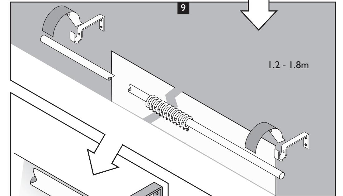
Centre the pole and tighten the locking screws on the brackets, Fig. 10.
