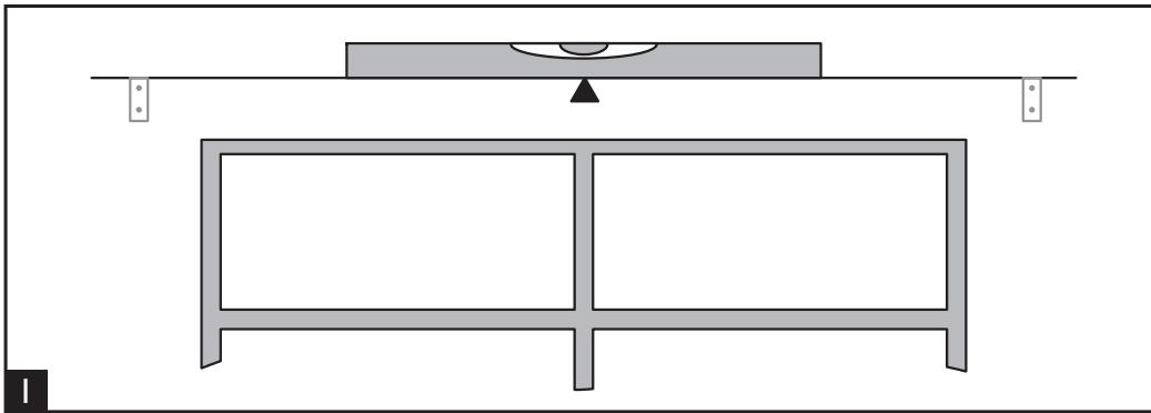
Use a spirit level to mark the top line of the brackets, Fig. 1. If you are mounting an additional intermediate bracket, space it evenly between the two outermost brackets.
