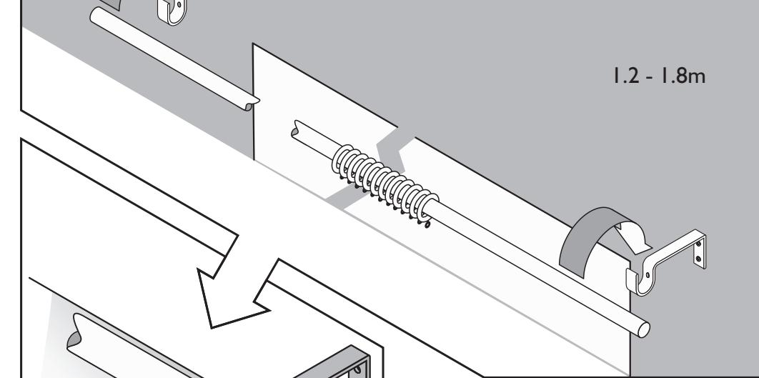
Centre the pole and tighten the locking screws on the brackets, Fig. 10.
