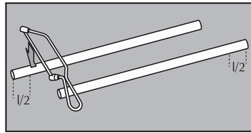
If it is necessary to shorten the pole, use a hacksaw to cut to the length required. Where there are two poles cut equal amounts off each pole.
