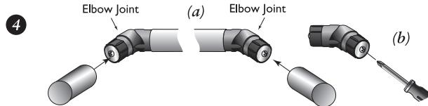
(a) Push the Elbow Joints securely into the ends of the poles.
