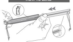
Lightly spray the inside of the track with silicon or furniture polish. Slide both the bending inserts into the track channel ensuring the flat edges are positioned together and the cords are at opposite ends as shown.
