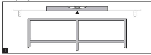
Use a spirit level to mark the top line of the brackets, Fig. 1. If you are mounting an additional intermediate bracket, space it evenly between the two outermost brackets.
