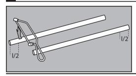
If it is necessary to shorten the pole, use a hacksaw to cut to the length required. Where there are two poles cut equal amounts off each pole.
